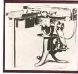
ILLUSTRATION OF THE ELECTRICALLY-OPERATED 'BICKERDIKE' POSTMARKING MACHINE HAVING THE ABILITY TO POSTMARK UP TO ABOUT 1000+ UNITS (HOW AT A COST TO THE REICHSPOST OF 225.00 RM/EACH MACHINE.
